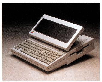
Inch and a quarter thick flat-screen display unit for the //c. Standard 24-line by 80-character screen display, including Hi-Res.
