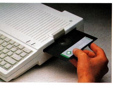
Built-in 5-1/4-inch "half high" disk drive. The unit is fully compatible with Apple's standard 35-track, 16-sector disk formats.
